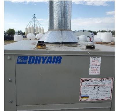
Figure 31 - HTF Fill Cap and Gauge
