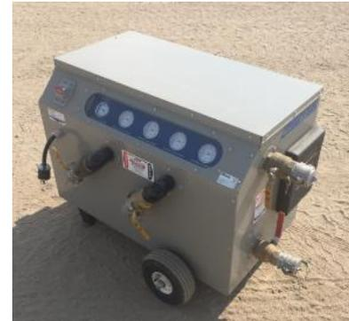
Figure 7 - Plate Heat Exchanger Unit
