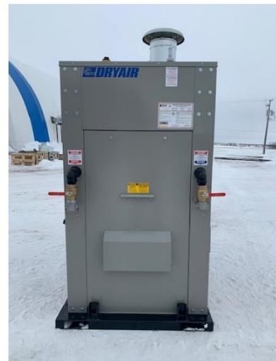
Figure 17 - Primary Circulation Line Connections
