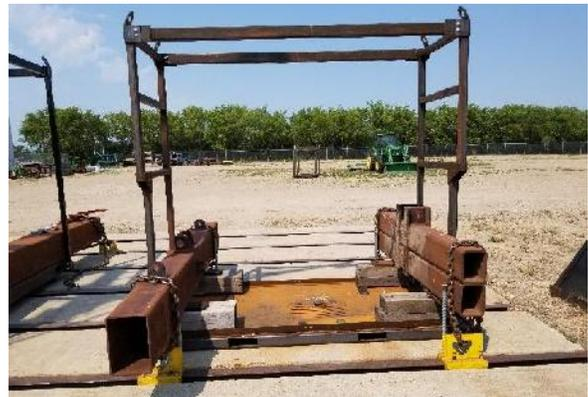
**Figure 1.** 2100x2 system base frame and installed lifting frame assembly secured to test bed.
