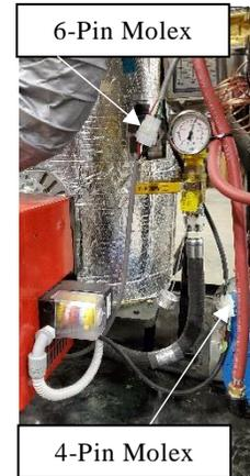
Figure 21 - Electrical Connection
